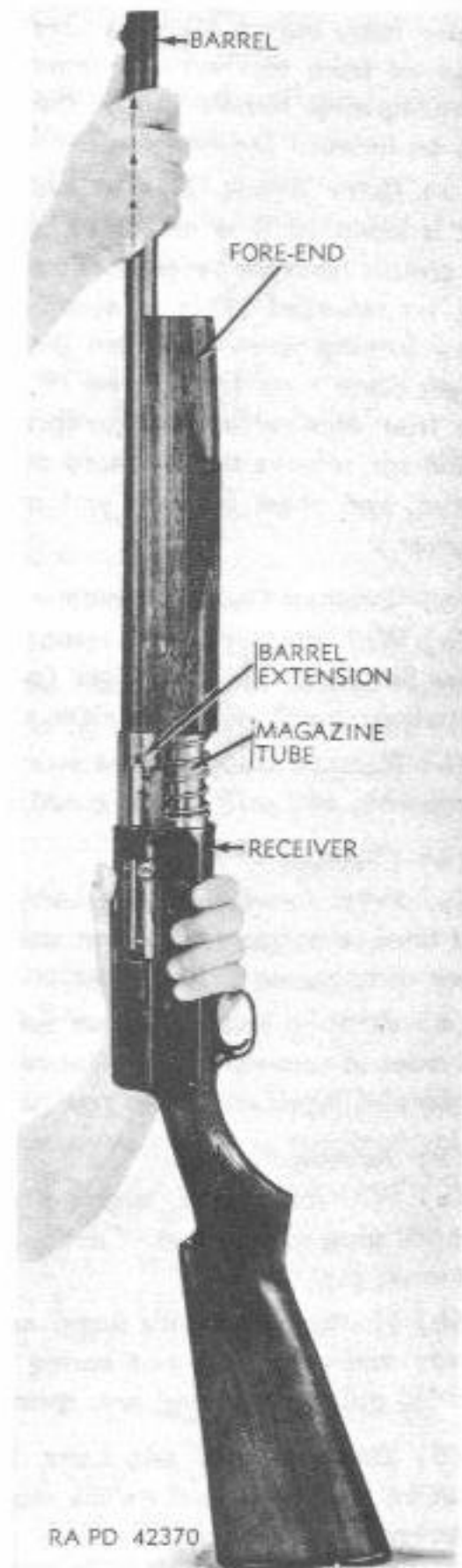
Figure 125—Easing Barrel (With Fore End) Out of Receiver—Savage Shotgun, M720
